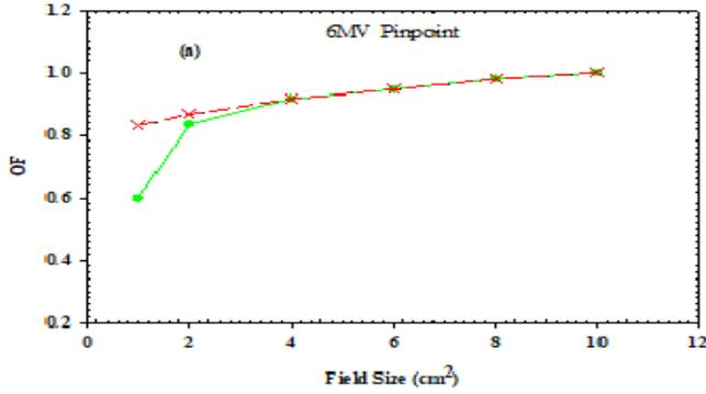
Figure 1: The Output Factor (OF) versus field size (cm<sup>2</sup>) for MLC/Jaw beams, 6MV beam energy using Pinpoint ion chamber. MLC (Red Cross-Red dash line), Jaw (Green Circle-Green Solid line).
