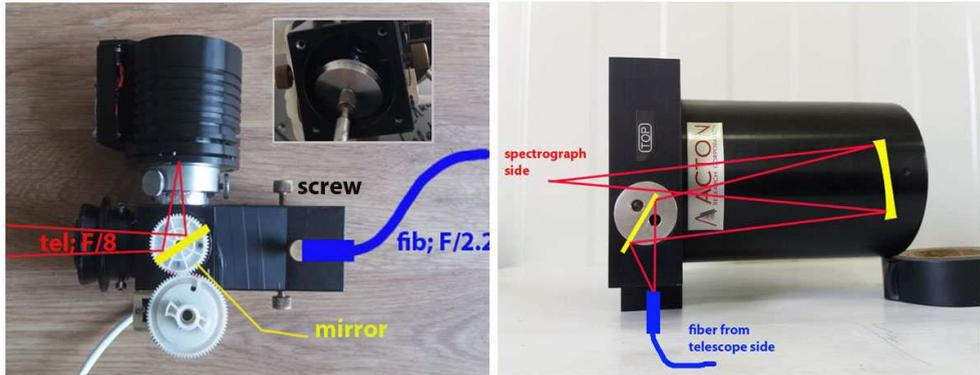
Figure 3: Instrument selector (left) and fibre coupler (right).
