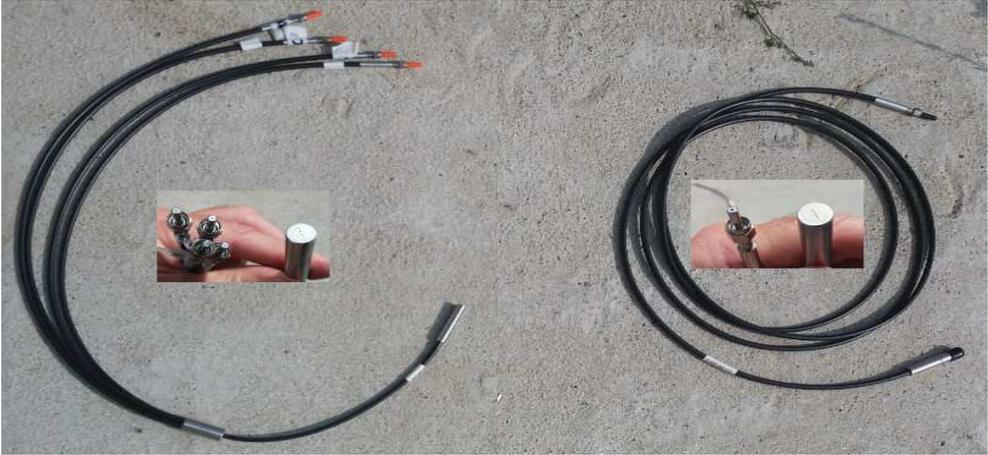
Figure 2: Two FOBs that were used with spectrograph: 4-legs FOB (left) and 1-leg FOB (right).
