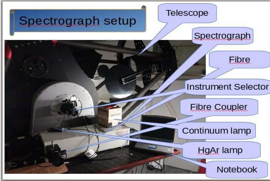
Figure 1: Spectrograph setup installed on the 1.4m telescope.
