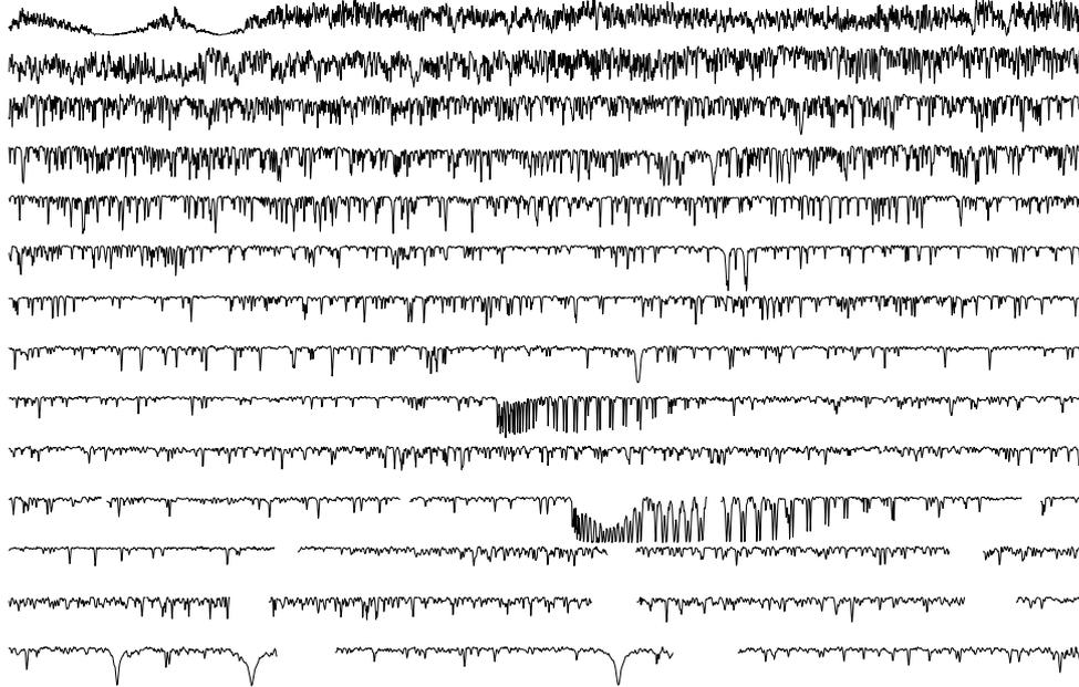
Figure 3: Example SES data: a full spectrum of HD 1. The wavelength coverage is from 390 to 870 nm, the gaps towards the red end of the spectrum are due to the comparably small format CCD detector in use until 2012.
