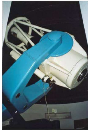
Figure 6: The 0.62m Ritchey-Chrétien telescope at OARMA.
