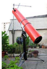
Newton telescope of the Society, apert. 23 cm
