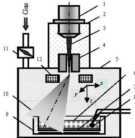
Figure 1: Scheme of the Electron-Beam Plasmachemical Reactor
