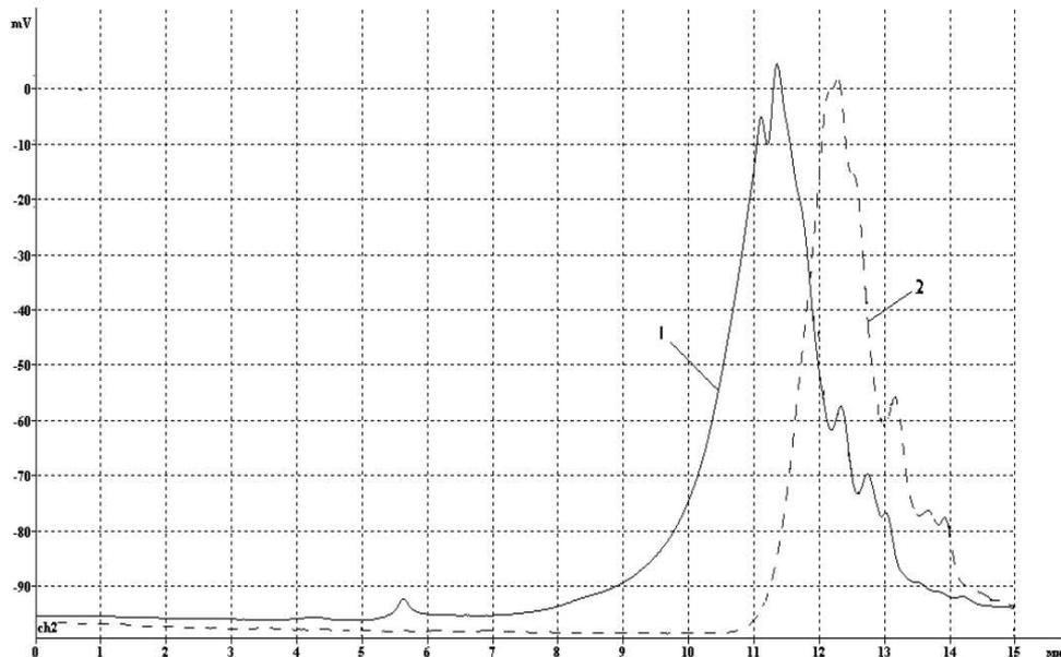
Figure 2: The chromatograms of the FM treated in the EBP of helium (1), water vapor (2).
