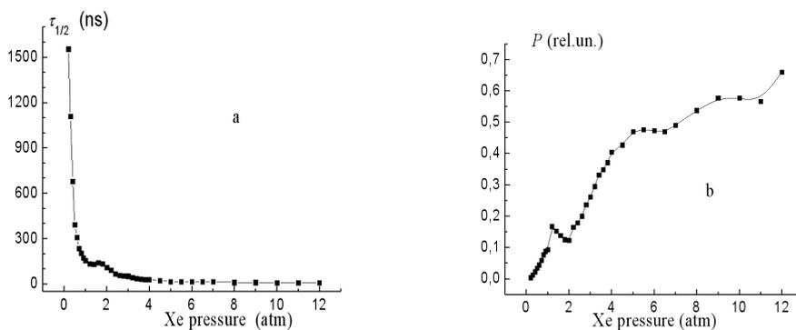
Figure 3: The duration (a) and power (b) of VUV radiation of Xe dimers vs Xe pressure.
