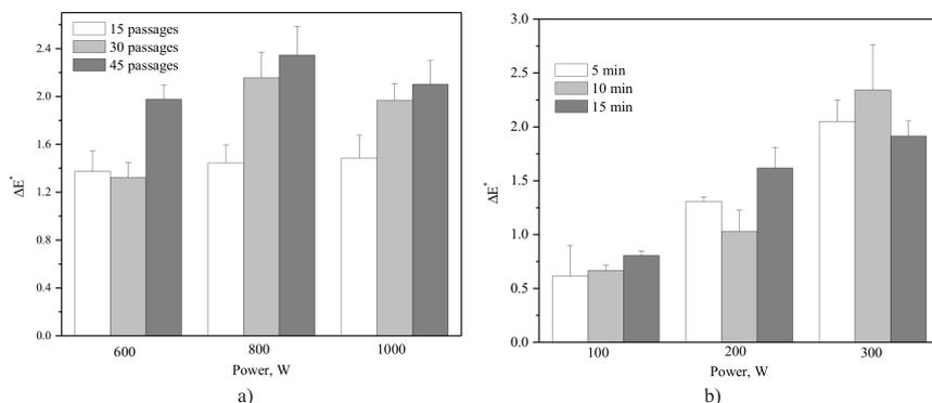
Figure 1: Colour difference ( $\Delta E^*$ ) after a) COR treatment and b) LPP treatment of denim.
