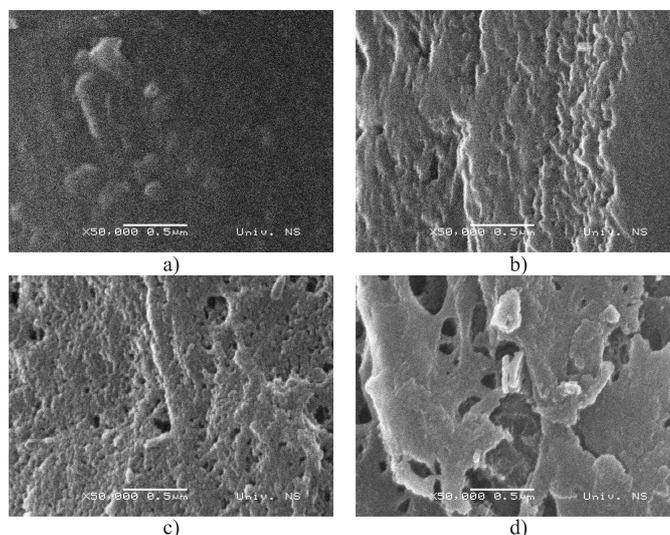
Figure 2: SEM images of a) untreated; b) corona treated (1000 W, 45 passages); c) argon LPP treated (300 W, 15 min) and air LPP treated (300 W, 15 min) fibres.
