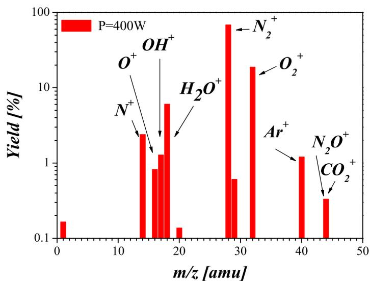
Figure 1: Mass to charge spectra for power of 400 W. Distance from the electrode from the mass analyzer was 5 mm.
