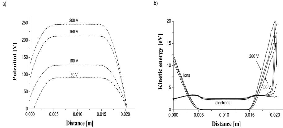
Figure 3: Changes of time-average: a) potential profile and b) kinetic energy, with the variation of the  $V_{\text{lf}}$  from 50 V to 200 V in DF-CCP (27MHz/2MHz) with a fixed  $V_{\text{hf}} = 400 \text{ V}$ .
