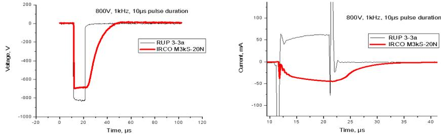
Figure 1: Voltage and current shapes during the pulse (the current of RUP3-3a is inverted for better presentation).
