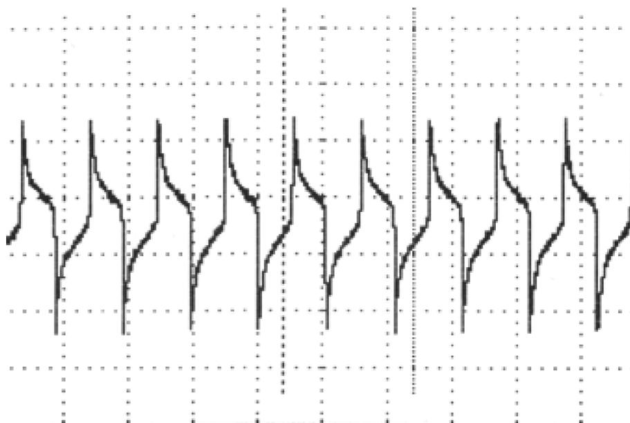
Figure 3: Oscillations under  $i = 1,5$  mA,  $\partial U/\partial i < 0$ .
