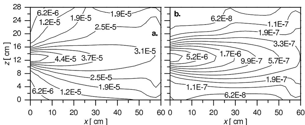
Figure 4: The relative density of a) O<sub>2</sub>(a) and b) O<sub>2</sub>(b) molecules in the reactor for  $x$ - $z$  vertical plane at  $y=15$  cm.
