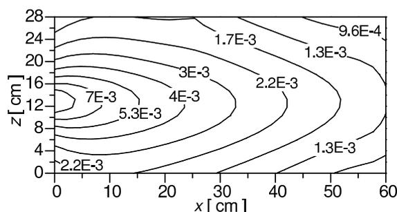
Figure 3: The relative density of O atoms in the reactor for  $x$ - $z$  vertical plane at  $y=15$  cm.
