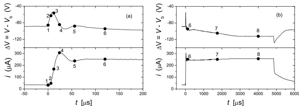
Figure 3: Voltage and current signals after the application of the voltage pulse: (a) beginning of the pulse zoomed in, (b) the whole pulse.
