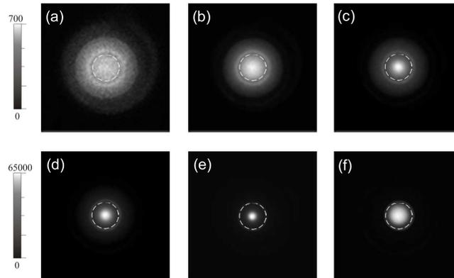
Figure 2: Radial profiles of the emission for different discharge currents: (a)  $i = 3.2 \mu\text{A}$ , (b)  $i = 28 \mu\text{A}$ , (c)  $i = 184 \mu\text{A}$ , (d)  $i = 231 \mu\text{A}$ , (e)  $i = 278 \mu\text{A}$ , (f)  $i = 4690 \mu\text{A}$ . White lines mark cathode cavity edge.
