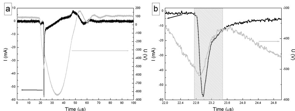
Figure 1: a) Applied voltage and discharge current variation during one cycle. Pressure 200 mbar.
