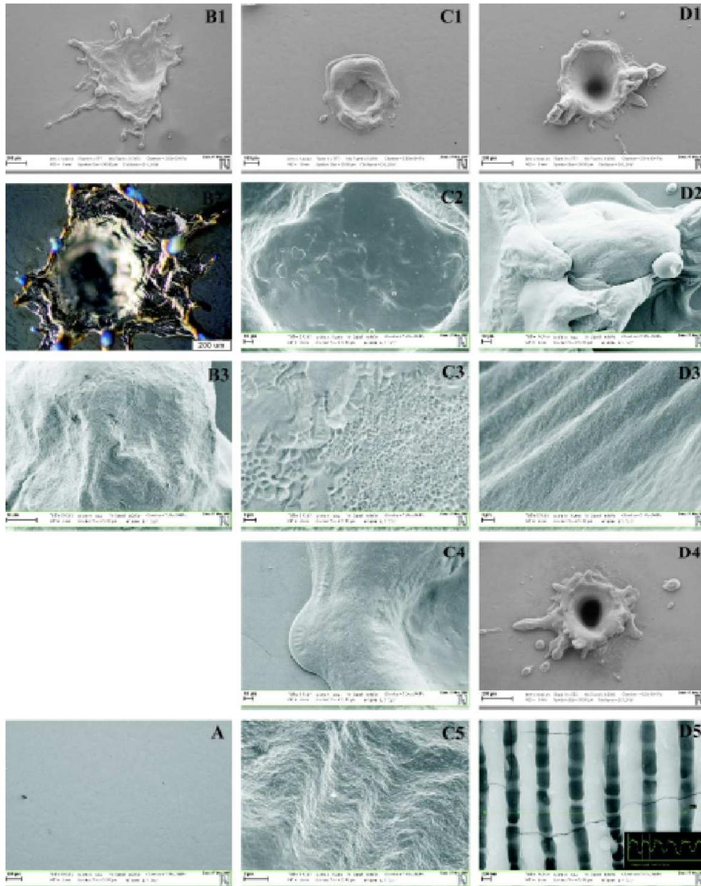
Figure 1: ps- Nd:YAG laser-induced Ti6Al4V implant morphology changes ( $\lambda=1064$  nm). (A) Prior and, (B), (C) after 1 laser pulse (different LPED). (D) After 5 and 100 laser pulses. LPED = 31.2 (B) and 23.6  $J/cm^2$  (C) and (D).
