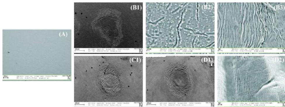
Figure 2: ps-Nd:YAG laser-induced Ti6Al4V implant morphology changes ( $\lambda=523$  nm). (A) Prior to laser action; (B) 1 laser pulse, (C) and (D) after 50 laser pulses. LPED = 25.9 J/cm<sup>2</sup>.
