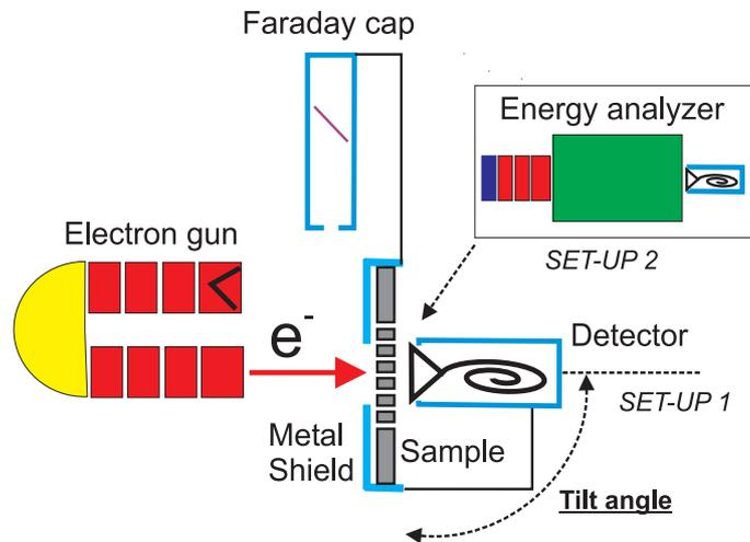
Figure 1: A schematic view of the experimental set-up.
