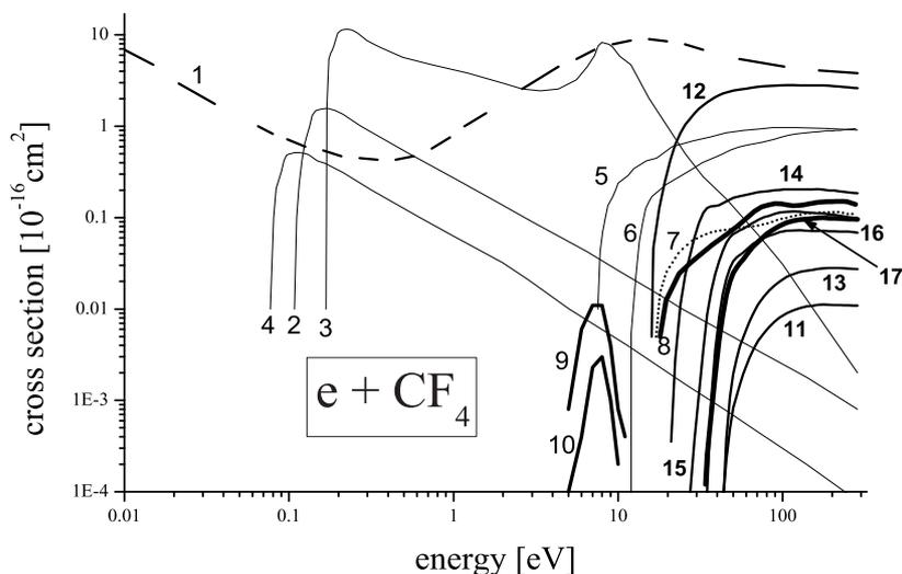
Figure 1: Electron impact cross sections for scattering on  $\text{CF}_4$  (1 - elastic momentum transfer, 2 - vibrational excitation  $v=1$ , 3 - vib. excitaton  $v=3$ , 4 - vib. excitation  $v=4$ , 5 - electron excitation, dissociation to products  $\text{CF}_3$  (6),  $\text{CF}_2$  (7),  $\text{CF}$  (8), 9 - dissociative electron attachment(DEA) ( $\text{F}^-$ ), 10 - DEA ( $\text{CF}_3^-$ ), 11 -  $\text{CF}_3^+ + \text{F} + 2e$  (ionization), 12-17 other channels of ionization).
