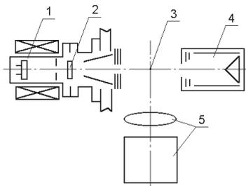
Figure 1: Experimental setup: 1 – ion source; 2 – multi-channel charge exchange cell; 3 – gas target; 4 – detector of fast atoms; 5 – optical recording system.
