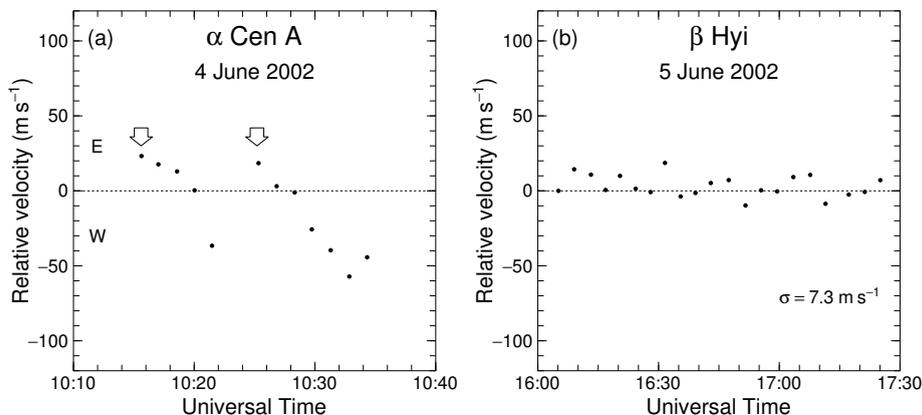
Figure 4: (a) The effect of poor scrambling by the optical fibre. The star drifts westward across the fibre while a sequence of observations is made. The telescope is repositioned only at the beginning of each sequence (as indicated by arrows). (b) Radial velocity of  $\beta$  Hyi over a short period of time. The star has been re-centred on the fibre before each exposure. Exposure time: 30–40 s.
