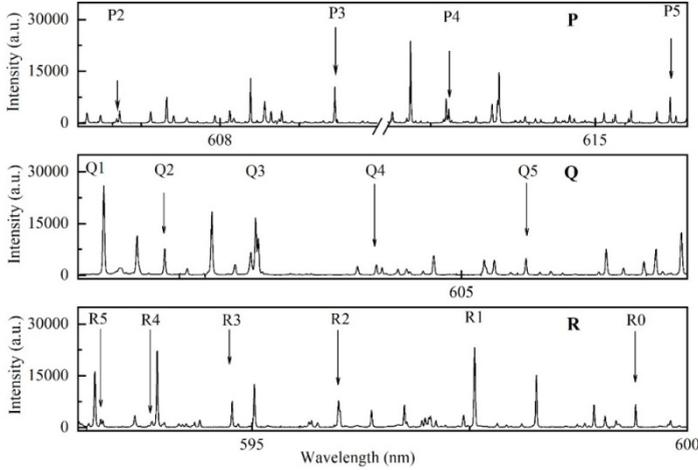
Figure 2: Emission spectra of the rotational lines for the  $d^3\Pi_u, v'=0 \rightarrow a^3\Sigma_g^+, v''=0$  band, P, Q and R-branches, recorded in the second order of diffraction grating. Experimental conditions: cooper cathode GDS in  $H_2+5\%Ar$  at  $p = 4.5$  mbar;  $I = 13.4$  mA;  $U = 646$  V.
