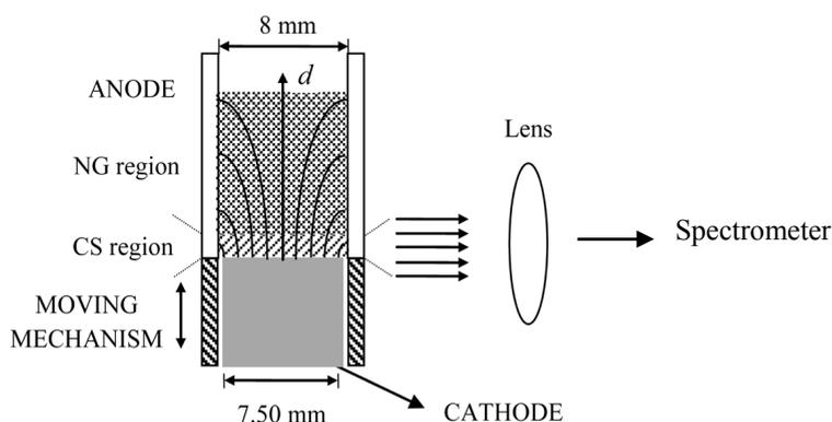
Figure 1: Schematic diagram of the central part of the Grimm GD for side-on observations. Symbols: CS – cathode sheath region, NG – negative glow region.
