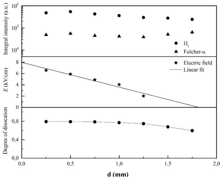
Figure 3: The dependence of: (a) Relative intensity of  $H_{\gamma}$  line and Fulcher- $\alpha$  bands ( $\nu'=\nu''=0, 1, 2, 3$ ) (b) Electric field strength and (c) Degree of dissociation, all upon the distance from the cathode. Experimental conditions: cooper cathode Grim GD in  $H_2+5\%Ar$  at  $p = 4.5$  mbar;  $I = 13.4$  mA;  $U = 646$  V.
