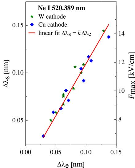
Figure 2. The side-on Stark shifts  $\Delta\lambda_s$  (and corresponding  $F_{\max}$ , Eq. 1) against the end-on Stark shifts  $\Delta\lambda_e$  for the spectral line Ne I 520.389 nm. Each point represents different discharge conditions (pressure, current, voltage), with either tungsten or copper cathodes.
