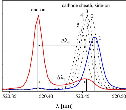
Figure 1. Ne I 520.389 nm spectral line recorded end-on (red line) and side-on in the CS at five different distances from the cathode (in 1/16 mm steps), starting from the maximum shift at  $F_{\max}$  (blue line). Measured shifts, end-on  $\Delta\lambda_e$ , and side-on  $\Delta\lambda_s$ , are indicated.
