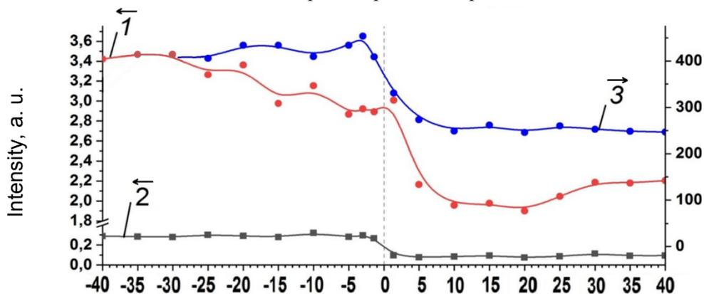
Fig. 4. – Dependence of line's intensity ratio Si II 385,6 / Si I 390,5 (1), Si III 380,6 / Si II 385,6 (2), Si II 385,6 / N II 501,1 (3) on time interval and order of laser pulses with wavelengths of 355 and 532 nm in silicon plasma
