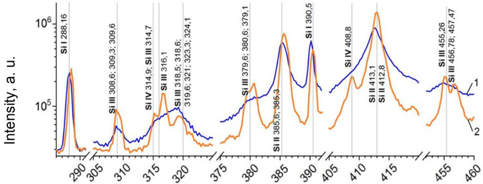
Fig. 2. – Spectra of surface plasma induced by monochromatic LI with  $\lambda=355$  nm and  $q_{355}=4,6$  GW/cm<sup>2</sup> (1) and bichromatic LI with  $q_{355}=1,9$  GW/cm<sup>2</sup> +  $q_{532}=3,5$  GW/cm<sup>2</sup> ( $\Delta\tau=1,4$   $\mu$ s) (2) on silicon sample in air
