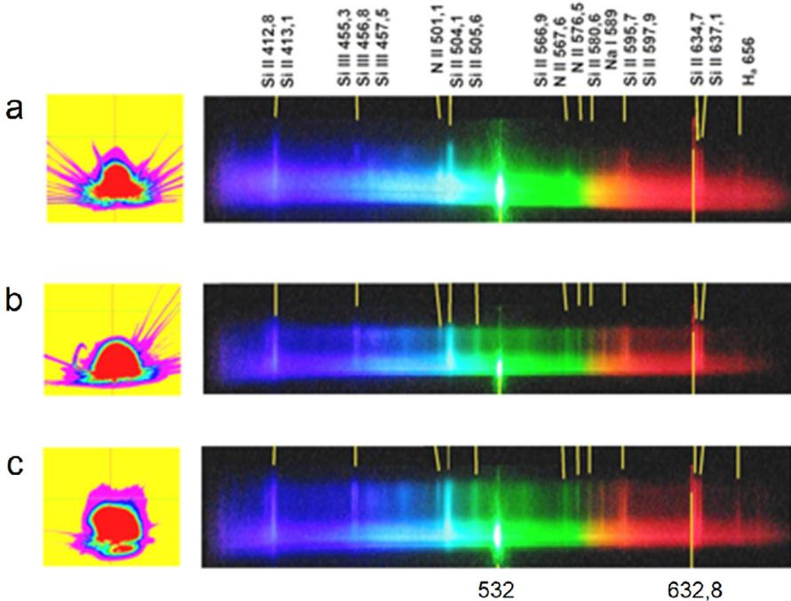
Fig. 3. – Video pictures of plasma plume and their corresponding spectra induced by bichromatic LI with  $q_{355}=1,9$  GW/cm<sup>2</sup> and  $q_{532}=3,5$  GW/cm<sup>2</sup> and interval between pulses  $\Delta\tau=-5,5$   $\mu$ s (a),  $-1,3$   $\mu$ s (b) and  $+15$   $\mu$ s (c).
