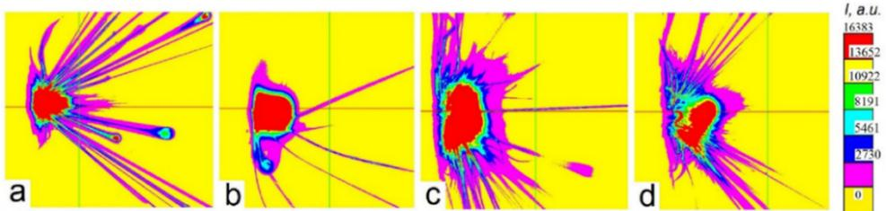
Fig. 1. – Video pictures of plasma plume induced by monochromatic (a, b) and bichromatic (c, d) laser irradiation on silicon: a –  $q_{355} = 1,9 \text{ GW}/\text{sm}^2$ , b –  $q_{532} = 3,5 \text{ GW}/\text{sm}^2$ ;
