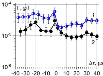
Figure 1: Dependences of the specific mass removal of silicon on the time interval within bichromatic laser pulses with power density  $q_{355} = 1.9$  and  $q_{532} = 3.5$   $\text{GW}/\text{cm}^2$  (1),  $q_{355} = 1.0$  and  $q_{532} = 1.94$   $\text{GW}/\text{cm}^2$  (2)
