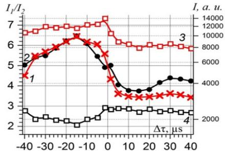
Figure 2: Ratio between the intensities of spectral lines Si II 412.9/N II 501.1 nm (1), Si II 412.9/Si I 288.2 nm (2), and dependences of the intensity of spectral line Si II 412.9 nm (3), N II 501.1 nm (4) on the time interval within bichromatic laser pulses with power density  $q_{355} = 1.9$  and  $q_{532} = 3.5$   $\text{GW}/\text{cm}^2$
