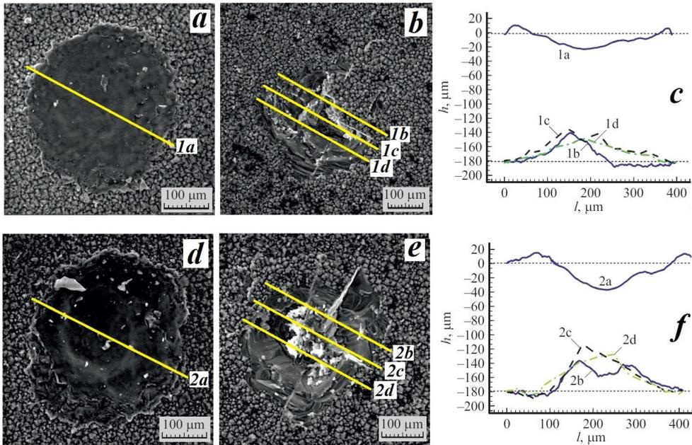
Figure 3: SEM images of ablation (a, d) and spallation (b, e) craters and the corresponding profiles (c, f), formed as a result of irradiation with four (a–c) and eight pairs (d–f) of laser pulses with wavelengths of 355 and 532 nm (treatment parameters:  $q_{355} = 1.9 \text{ GW/cm}^2$ ,  $q_{532} = 3.5 \text{ GW/cm}^2$ ,  $\Delta\tau = -3 \mu\text{s}$ ).
