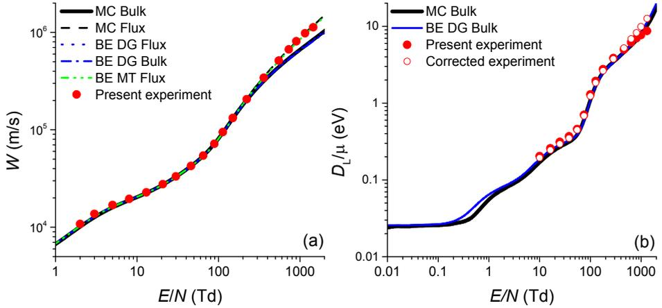
Figure 1: Comparison of the calculated flux and bulk drift velocities and the present experimental data (a), and comparison between the calculated bulk values of the longitudinal characteristic energy and the corrected and uncorrected experimental data (b).
