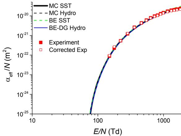
Figure 2: Variation of the density-reduced effective Townsend ionization coefficient with  $E/N$ .
