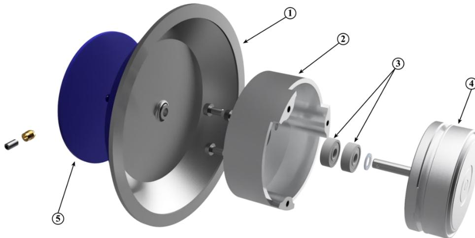
Figure 5: Exploded View of the Reaction Wheel Assembly: 1 – Rotor, 2 – Mounting Bracket, 3 – Bearings, 4 – Motor, 5 – Adapter Disk
