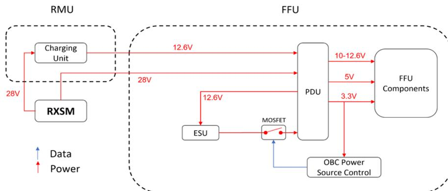
Figure 7: EPS Block Diagram
