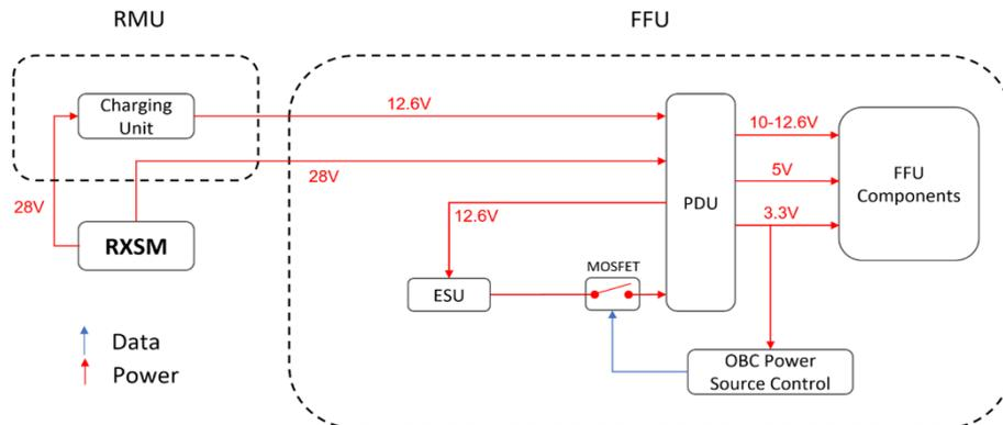
Figure 7: EPS Block Diagram
