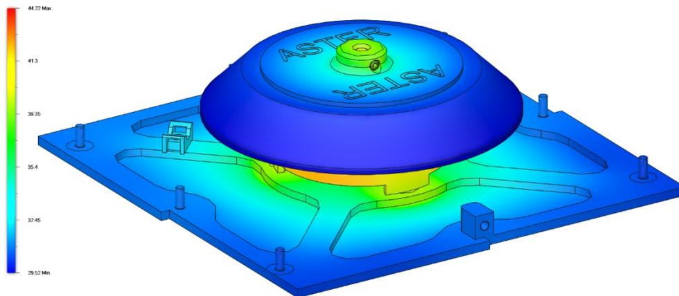
Figure 9: FEA of Reaction wheel showing temperature distribution.
