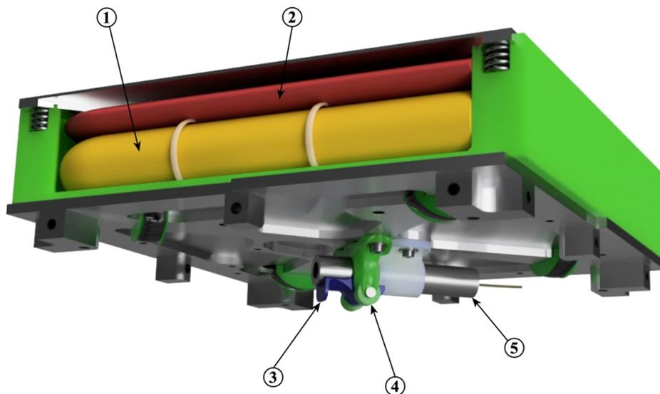
Figure 6: Recovery Compartment: 1 – Parachute, 2 – Streamer, 3 – Spark Cover, 4 – Retention Bracket, 5 – Pyro Cutter
