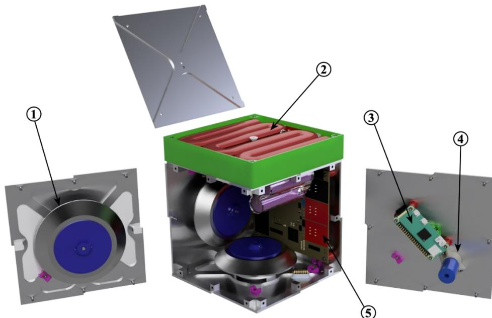
Figure 2: Open View of the Free Falling Unit: 1 – Reaction Wheel, 2 – Parachute, 3 – Payload, 4 – Iridium Antenna, 5 – Main PCB.
