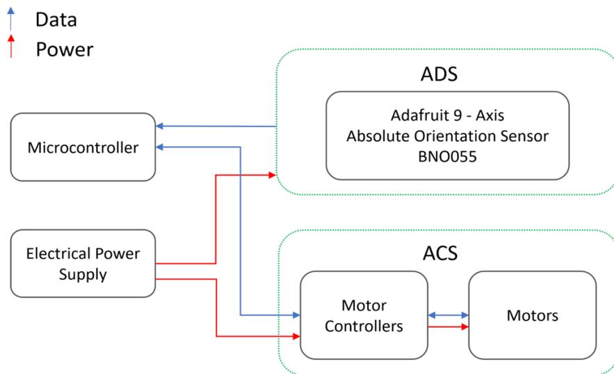
Figure 4: Schematics of the Attitude Determination and Control System Electronic Design.
