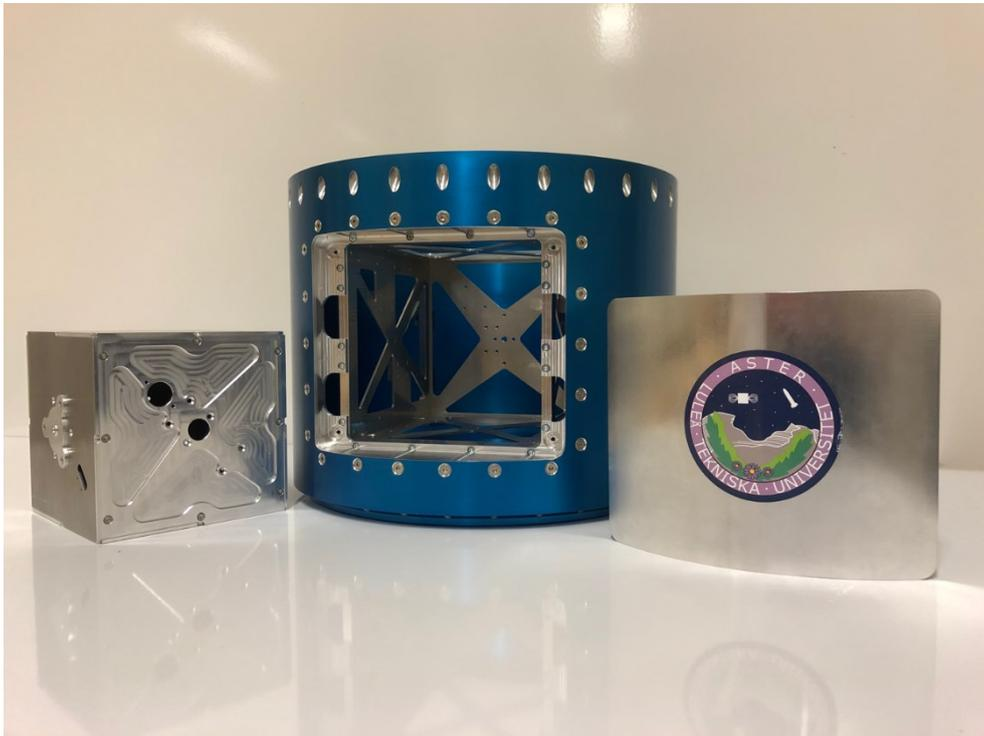
Figure 11: The FFU and the RMU inside the Experiment Module.
