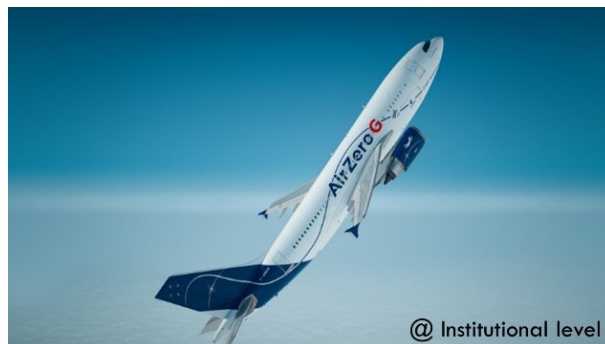
Image 3: The Airbus 310 of the French company NOVESPACE injects into the 43-degree flight path for flying along a parabolic arc. Credit: NOVESPACE
