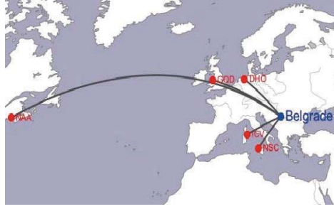
Figure 1: The geographic position of Belgrade system of VLF/LF receivers and the surrounding transmitters.
