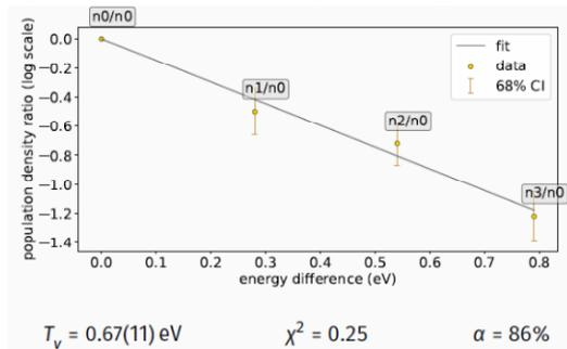
Figure 4: Extraction of the excitation temperature of the  $H_2$  3c state in the cell corresponding to the brighter spot of the plasma column.
