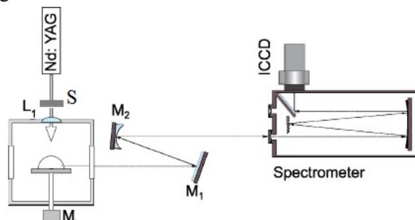
Figure 1: LIBS setup
