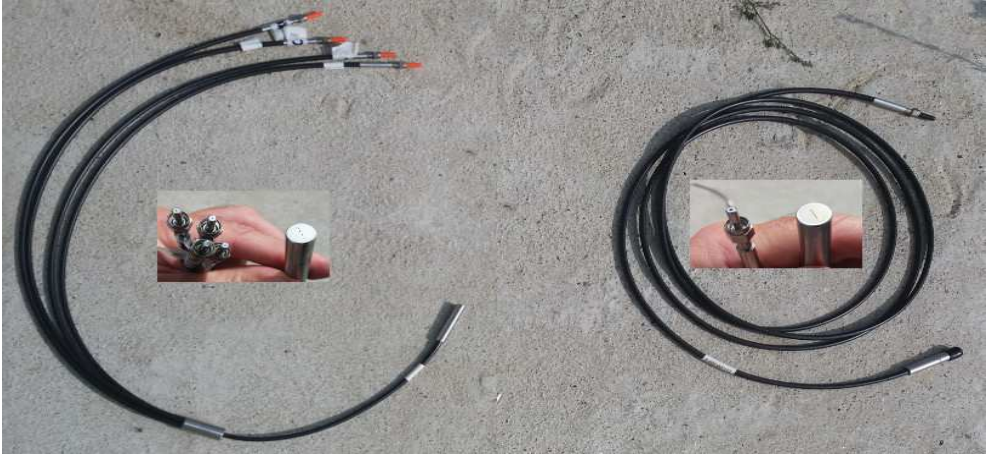
Figure 2: Two FOBs that were used with spectrograph: 4-legs FOB (left) and 1-leg FOB (right).
