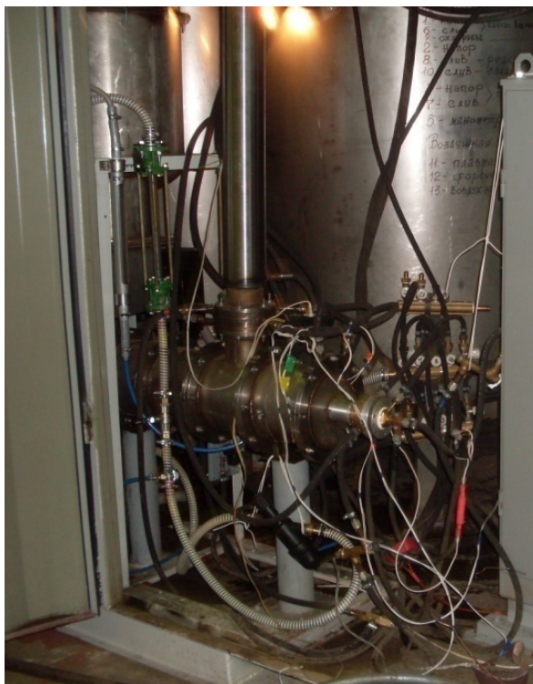
Figure 3: Counterflow plasma reactor with plasma torch PDS-3/50.
