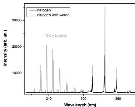
**Figure 6:** Emission spectra from coaxial DBD in nitrogen and nitrogen with water.
