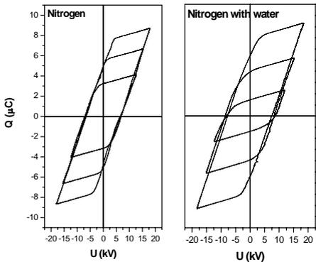
**Figure 4:** Lissajous figures obtained for different applied voltages for coaxial DBD in nitrogen and nitrogen with water.
