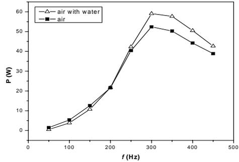
**Figure 3:** The effect of applied frequency on discharge power in air and air with water.
