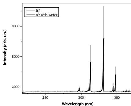
**Figure 7:** Emission spectra from coaxial DBD in air and air with water.
