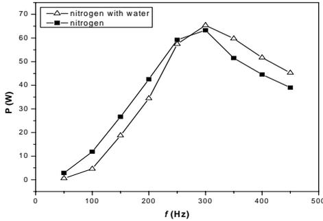
**Figure 2:** The effect of applied frequency on discharge power in nitrogen and nitrogen with water.
