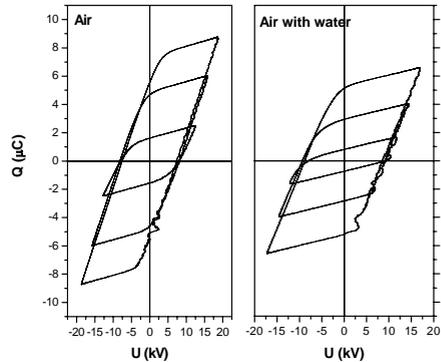
**Figure 5:** Lissajous figures obtained for different applied voltages for coaxial DBD in air and air with water.
