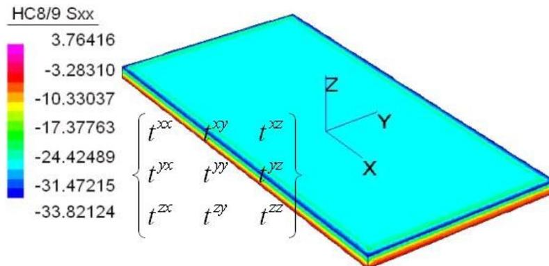
Figure 3: Fixed plate loaded by temperature gradient through its thickness. FE HC9/9 (full theory).
