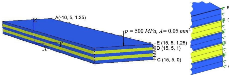
Figure 4: Composite Strip under midspan continual load.
