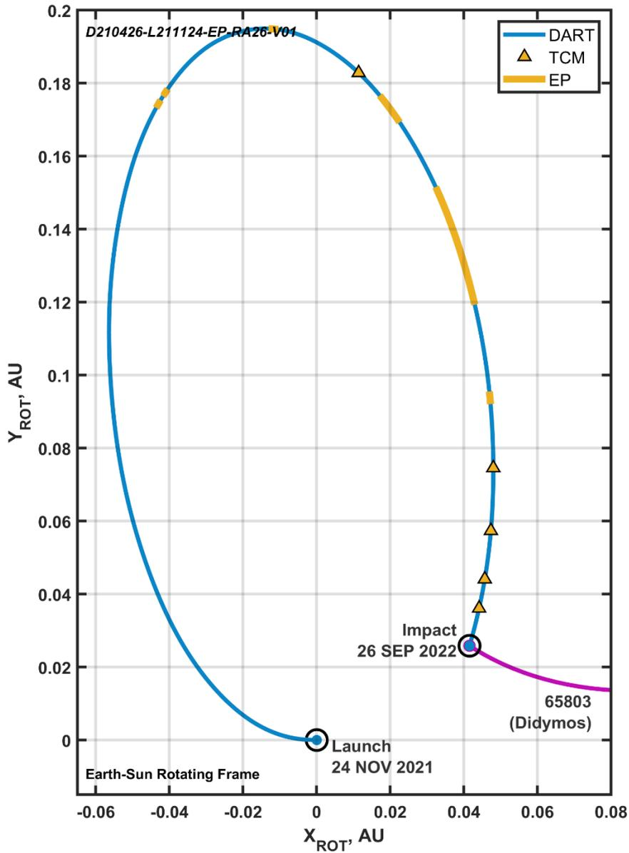
Figure 4: DART’s launch period open trajectory, shown in X-Y axes of an Earth-Sun rotating frame.
