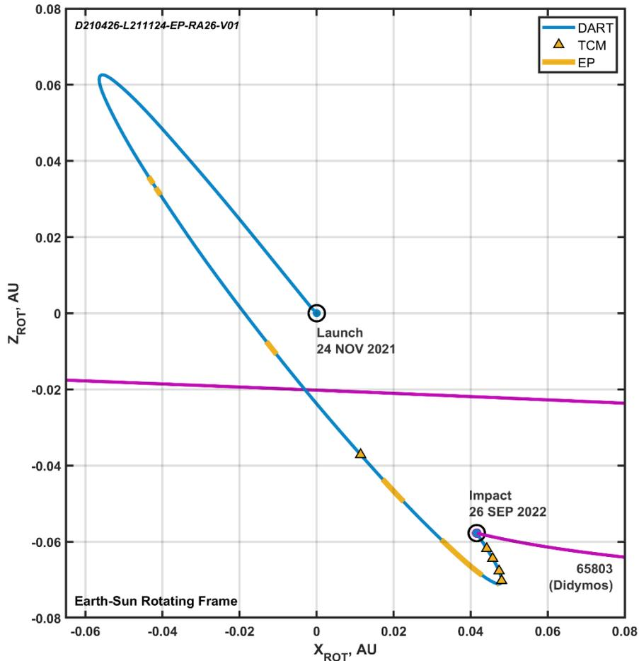
Figure 5: DART's launch period open trajectory, shown in X-Z axes of an Earth-Sun rotating frame.
