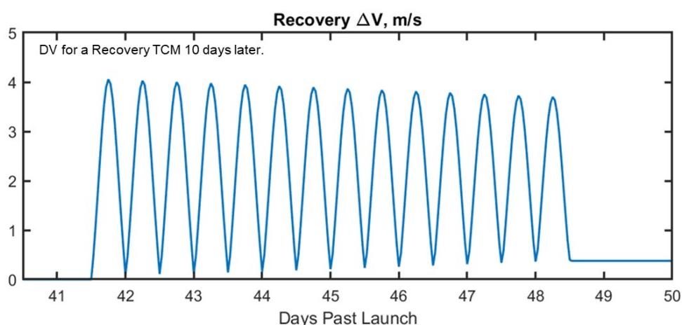
Figure 6: Recovery  $\Delta V$  cost for a maneuver conducted 10 days following a neutral burn failure.
